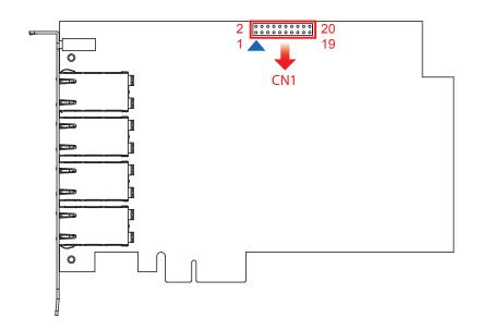
The PE-1000 offers a 16-bit Isolated DIO (8-DI / 8-DO) connector. Each bit of DI and DO equipped with a photo-coupler for protection. A power buffer device TPD2007F integrated in 8-DO circuit for industrial applications.
