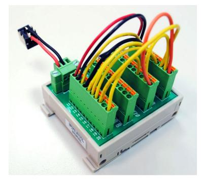
d. Connect 24V to Terminal board
