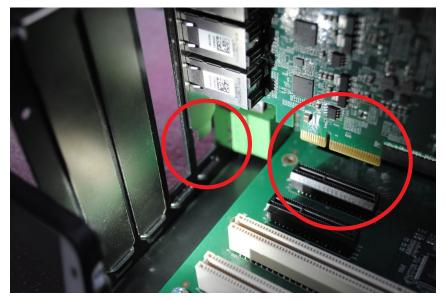
**Step 2.** Make sure golden finger and PCI bracket was inserted smoothly.
