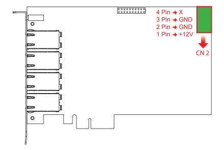
The PE-1000 also equipped with one 4-pin power plug (12V, 6A max) for additional power supply. For most cases, the power obtained from PCIe bus is sufficient for the PoE devices, and you do not need to supply extra power to the card.
