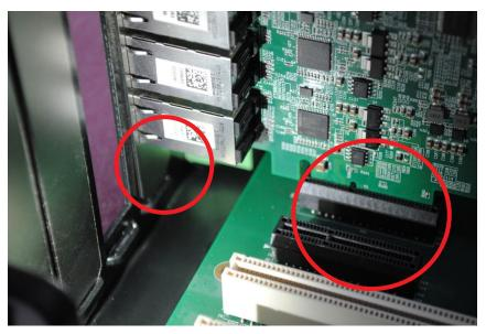
**Step 3.** Make sure the bracket aligns screw hole.
