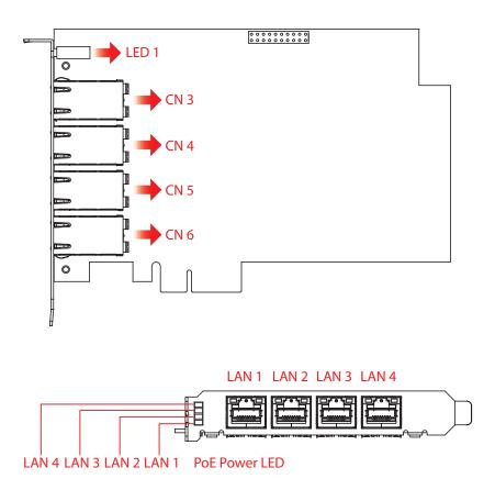
PE-1000 equipped with 4 IEEE 802.3at PoE<sup>+</sup> ports for transmitting power as much as 25.5W / 48V per port and 1000BASE-T gigabit data signals over standard Ethernet CAT-5/CAT-6 cable. Every PoE port applies one Intel<sup>®</sup> 82574L Gigabit Ethernet controller and independent PCI express interface to connect with multi-core processor for network and data transmit optimization. Only when PoE port starts to supply power to power devices, the dedicated LED will be light on.
